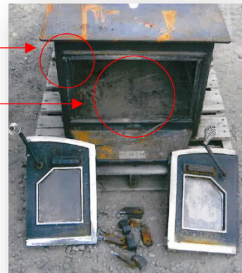
C. Front of the appliance showing that the door and firebrick were removed and that the door hinge mechanism was smashed
